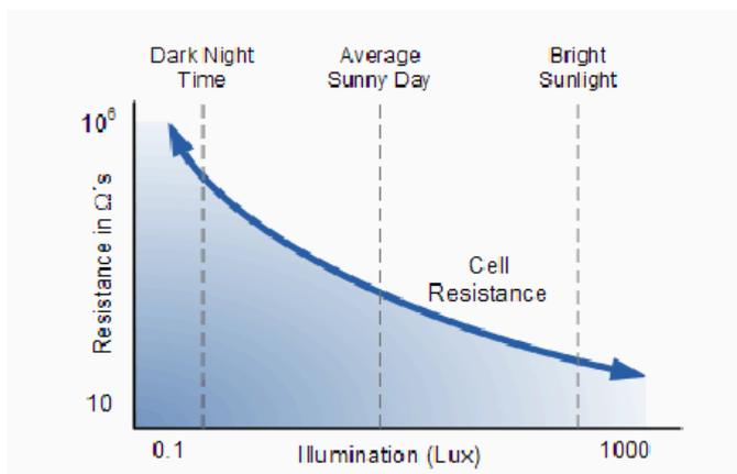
**Fig -6** Experimental Result of LDR
