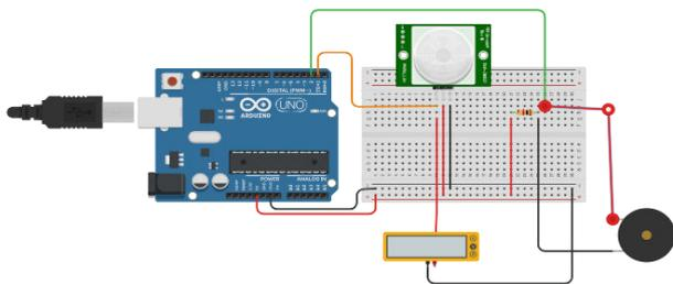
Fig -8 Arduino Interface with PIR motion sensor through buzzer and LCD display
