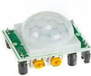
Fig -7 PIR Motion Sensor
